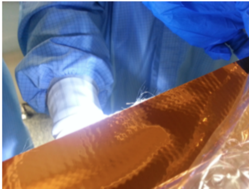
A flight-spare blanket of the Gaia sun shield lit with a torch from the back to enhance the effect of scattered light from fibres protruding from the edge.
