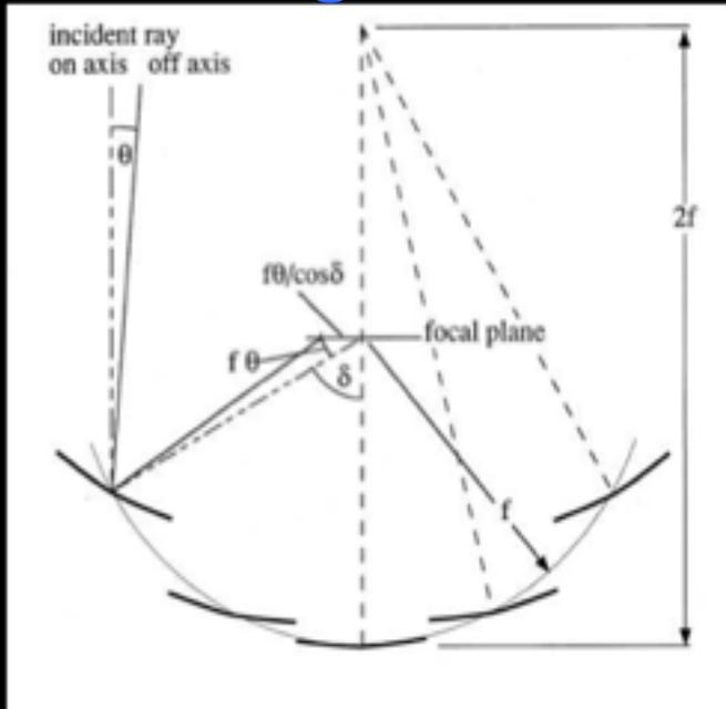
The **facets** are manufactured as spherical mirrors and arranged in a Davies-Cotton layout, in which all reflector facets have the same **focal length  $f$** , which is identical to the focal length of the telescope as a whole. The facets are arranged on a sphere with a radius of  $2f$ . Such an arrangement was chosen because of the cost and optical error reasons.
